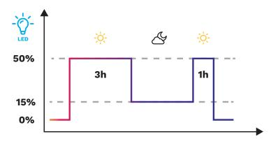
At nightfall, the luminaire is switched on at 50% of its maximum output for 3 hours. It then reduces its output to 15% to provide safety lighting throughout the night. At sunrise, the light output returns to 50% for one hour before the luminaires switch off.
