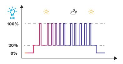
At nightfall, the luminaire is switched on at 20% of its maximum output for the whole night. When movement is detected (car, bicycle or pedestrian), the lighting level is temporarily increased to 100% to provide maximum safety and comfort to users. This dimming profile allows up to 450 detections per night.
