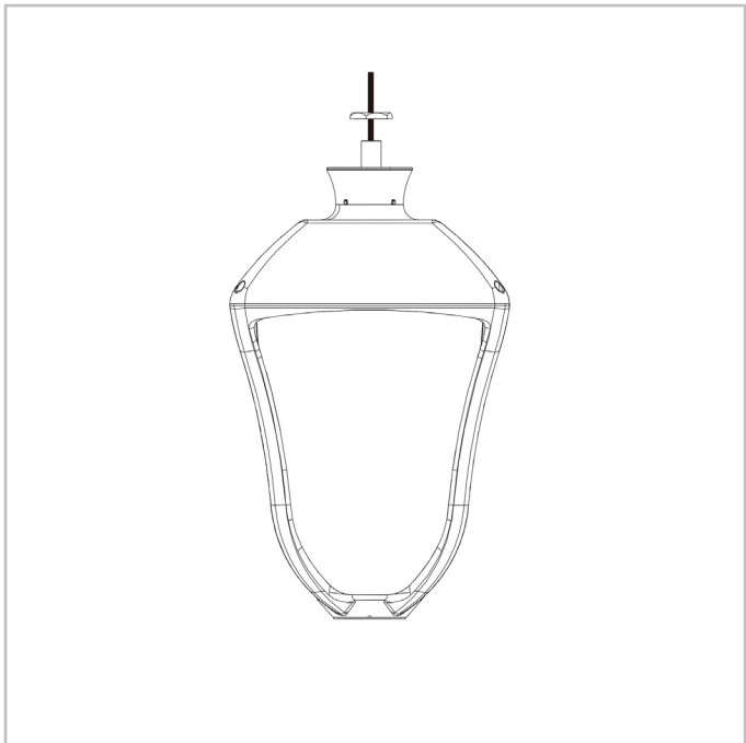
STYLAGE | Suspended mounting with a 1 inch female or 3/4 inch gas fixation
