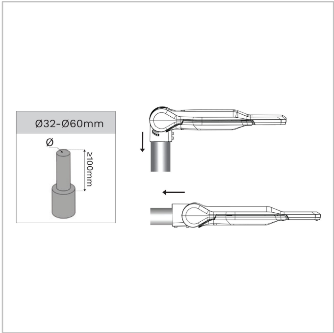
IZYLUM NEO | Slip-over mounting for Ø32-60mm spigot - 2xM10 screws
