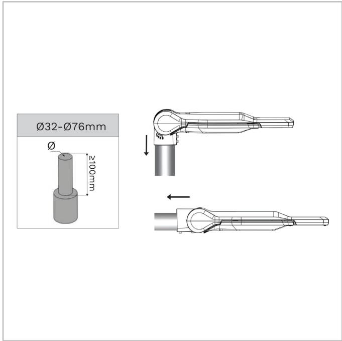
IZYLUM NEO | Slip-over mounting for Ø32-76mm spigot - 2xM10 screws
